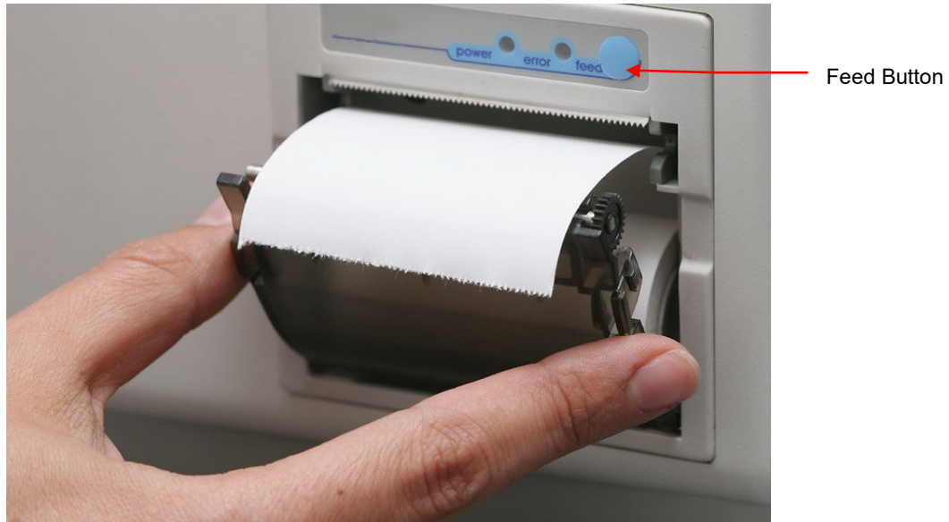
Figure 48 - Insert Paper Roll into printer
